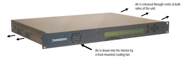
Figure 2.1: Air flow Through the Equipment
